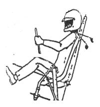
The shoulder harness should be mounted behind the driver and above a line drawn downward from the shoulder point at an angle of 40 degrees with the horizontal.
