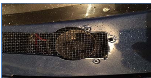
Figure 1 Rectangle 13 ⅛" x 2 ⅛" opening below the windshield (allowed on both original body and 2006 body)
